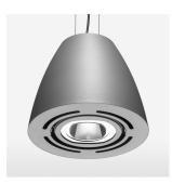
Suspended luminaire with LED, rated life of the LED L80/B10 > 50000 h, colour rendering index CRI > 80, chromaticity tolerance 2 SDCM (initial), reflector with circular light distribution pattern, reflector pure aluminium 99,99% in MIRO-Silver®, swivel angle 2x25°, luminaire housing sheet steel, powder-coated, stratosilver
