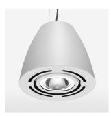
Suspended luminaire with LED, rated life of the LED L80/B10 > 50000 h, colour rendering index CRI > 90, chromaticity tolerance 2 SDCM (initial), reflector with circular light distribution pattern, reflector pure aluminium 99,99% in MIRO-Silver®, swivel angle 2x25°, luminaire housing sheet steel, powder-coated, stratowhite
