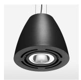
Suspended luminaire with LED, rated life of the LED L80/B10 > 50000 h, chromaticity tolerance 3 SDCM (initial), reflector with circular light distribution pattern, reflector pure aluminium 99,99% in MIRO-Silver®, swivel angle  $2x25^\circ$ , luminaire housing sheet steel, powder-coated, stratoblack
