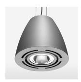
Suspended luminaire with LED, rated life of the LED L80/B10 > 50000 h, colour rendering index CRI > 90, chromaticity tolerance 2 SDCM (initial), reflector with circular light distribution pattern, reflector pure aluminium 99,99% in MIRO-Silver®, swivel angle 2x25°, luminaire housing sheet steel, powder-coated, stratosilver
