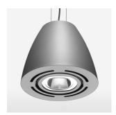
Suspended luminaire with LED, rated life of the LED L80/B10 > 50000 h, chromaticity tolerance 3 SDCM (initial), reflector with circular light distribution pattern, reflector pure aluminium 99,99% in MIRO-Silver®, swivel angle  $2x25^\circ$ , luminaire housing sheet steel, powder-coated, stratosilver
