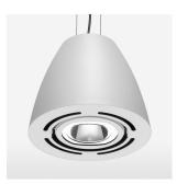
Suspended luminaire with LED, rated life of the LED L80/B10 > 50000 h, chromaticity tolerance 3 SDCM (initial), reflector with circular light distribution pattern, reflector pure aluminium 99,99% in MIRO-Silver®, swivel angle 2x25°, luminaire housing sheet steel, powder-coated, stratowhite
