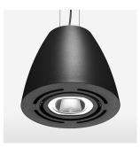
Suspended luminaire with LED, rated life of the LED L80/B10 > 50000 h, chromaticity tolerance 2 SDCM (initial), reflector with circular light distribution pattern, reflector pure aluminium 99,99% in MIRO-Silver®, swivel angle 2x25°, luminaire housing sheet steel, powder-coated, stratoblack
