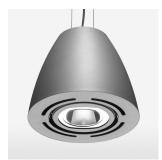
Suspended luminaire with LED, rated life of the LED L80/B10 > 50000 h, chromaticity tolerance 2 SDCM (initial), reflector with circular light distribution pattern, reflector pure aluminium 99,99% in MIRO-Silver®, swivel angle  $2x25^\circ$ , luminaire housing sheet steel, powder-coated, stratosilver
