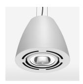
Suspended luminaire with LED, rated life of the LED L80/B10 > 50000 h, colour rendering index CRI > 90, chromaticity tolerance 2 SDCM (initial), reflector with circular light distribution pattern, reflector pure aluminium 99,99% in MIRO-Silver®, swivel angle 2x25°, luminaire housing sheet steel, powder-coated, stratowhite
