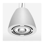
Suspended luminaire with LED, rated life of the LED L80/B10 > 50000 h, colour rendering index CRI > 90, chromaticity tolerance 2 SDCM (initial), reflector with oval light distribution pattern, reflector pure aluminium 99,99% in MIRO-Silver®, swivel angle  $2 \times 25^\circ$ , luminaire housing sheet steel, powder-coated, stratowhite
