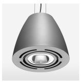
Suspended luminaire with LED, rated life of the LED L80/B10 > 50000 h, chromaticity tolerance 2 SDCM (initial), reflector with oval light distribution pattern, reflector pure aluminium 99,99% in MIRO-Silver®, swivel angle 2x25°, luminaire housing sheet steel, powder-coated, stratosilver
