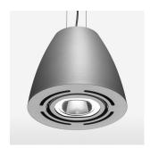
Suspended luminaire with LED, rated life of the LED L80/B10 > 50000 h, chromaticity tolerance 3 SDCM (initial), reflector with oval light distribution pattern, reflector pure aluminium 99,99% in MIRO-Silver®, swivel angle 2x25°, luminaire housing sheet steel, powder-coated, stratosilver
