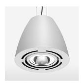
Suspended luminaire with LED, rated life of the LED L80/B10 > 50000 h, chromaticity tolerance 3 SDCM (initial), reflector with oval light distribution pattern, reflector pure aluminium 99,99% in MIRO-Silver®, swivel angle 2x25°, luminaire housing sheet steel, powder-coated, stratowhite
