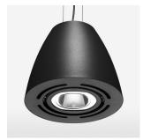
Suspended luminaire with LED, rated life of the LED L80/B10 > 50000 h, chromaticity tolerance 2 SDCM (initial), reflector with oval light distribution pattern, reflector pure aluminium 99,99% in MIRO-Silver®, swivel angle 2x25°, luminaire housing sheet steel, powder-coated, stratoblack
