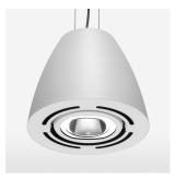
Suspended luminaire with LED, rated life of the LED L80/B10 > 50000 h, colour rendering index CRI > 90, chromaticity tolerance 2 SDCM (initial), reflector with oval light distribution pattern, reflector pure aluminium 99,99% in MIRO-Silver®, swivel angle 2x25°, luminaire housing sheet steel, powder-coated, stratowhite
