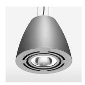
Suspended luminaire with LED, rated life of the LED L80/B10 > 50000 h, chromaticity tolerance 2 SDCM (initial), reflector with oval light distribution pattern, reflector pure aluminium 99,99% in MIRO-Silver®, swivel angle  $2x25^{\circ}$ , luminaire housing sheet steel, powder-coated, stratosilver
