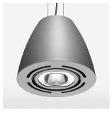
Suspended luminaire with LED, rated life of the LED L80/B10 > 50000 h, chromaticity tolerance 3 SDCM (initial), reflector with oval light distribution pattern, reflector pure aluminium 99,99% in MIRO-Silver®, swivel angle 2x25°, luminaire housing sheet steel, powder-coated, stratosilver
