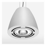
Suspended luminaire with LED, rated life of the LED L80/B10 > 50000 h, chromaticity tolerance 3 SDCM (initial), reflector with circular light distribution pattern, reflector pure aluminium 99,99% in MIRO-Silver®, swivel angle  $2 \times 25^\circ$ , luminaire housing sheet steel, powder-coated, stratowhite
