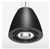
Suspended luminaire with LED, rated life of the LED L80/B10 > 50000 h, chromaticity tolerance 3 SDCM (initial), reflector with circular light distribution pattern, reflector pure aluminium 99,99% in MIRO-Silver®, swivel angle  $2x25^\circ$ , luminaire housing sheet steel, powder-coated, stratoblack
