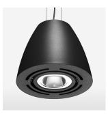
Suspended luminaire with LED, rated life of the LED L80/B10 > 50000 h, chromaticity tolerance 3 SDCM (initial), reflector with circular light distribution pattern, reflector pure aluminium 99,99% in MIRO-Silver®, swivel angle 2x25°, luminaire housing sheet steel, powder-coated, stratoblack
