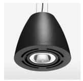
Suspended luminaire with LED, rated life of the LED L80/B10 > 50000 h, chromaticity tolerance 2 SDCM (initial), reflector with circular light distribution pattern, reflector pure aluminium 99,99% in MIRO-Silver®, swivel angle  $2 \times 25^\circ$ , luminaire housing sheet steel, powder-coated, stratoblack
