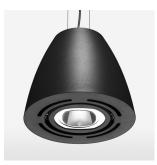
Suspended luminaire with LED, rated life of the LED L80/B10 > 50000 h, colour rendering index CRI > 90, chromaticity tolerance 2 SDCM (initial), reflector with circular light distribution pattern, reflector pure aluminium 99,99% in MIRO-Silver®, swivel angle 2x25°, luminaire housing sheet steel, powder-coated, stratoblack
