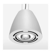
Suspended luminaire with LED, rated life of the LED L80/B10 > 50000 h, chromaticity tolerance 2 SDCM (initial), reflector with oval light distribution pattern, reflector pure aluminium 99,99% in MIRO-Silver®, swivel angle 2x25°, luminaire housing sheet steel, powder-coated, stratowhite
