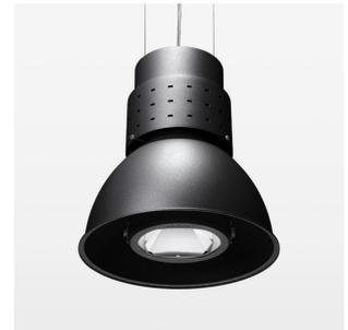
Suspended luminaire with LED, rated life of the LED L80/B10 > 50000 h, chromaticity tolerance 2 SDCM (initial), reflector with circular light distribution pattern, reflector pure aluminium 99,99% in MIRO-Silver®, luminaire shade die-cast aluminium, powder-coated, swivel angle +25°/-25°, luminaire housing sheet steel, powder-coated, stratoblack
