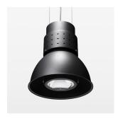
Suspended luminaire with LED, rated life of the LED L80/B10 > 50000 h, chromaticity tolerance 2 SDCM (initial), reflector with circular light distribution pattern, reflector pure aluminium 99,99% in MIRO-Silver®, luminaire shade die-cast aluminium, powder-coated, swivel angle +25°/-25°, luminaire housing sheet steel, powder-coated, stratoblack
