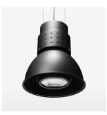
Suspended luminaire with LED, rated life of the LED L80/B10 > 50000 h, chromaticity tolerance 2 SDCM (initial), reflector with oval light distribution pattern, reflector pure aluminium 99,99% in MIRO-Silver®, luminaire shade die-cast aluminium, powder-coated, swivel angle +25°/-25°, luminaire housing sheet steel, powder-coated, stratoblack
