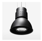
Suspended luminaire with LED, rated life of the LED L80/B10 > 50000 h, chromaticity tolerance 3 SDCM (initial), reflector with oval light distribution pattern, reflector pure aluminium 99,99% in MIRO-Silver®, luminaire shade die-cast aluminium, powder-coated, swivel angle +25°/-25°, luminaire housing sheet steel, powder-coated, stratoblack
