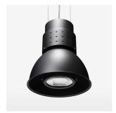
Suspended luminaire with LED, rated life of the LED L80/B10 > 50000 h, chromaticity tolerance 3 SDCM (initial), reflector with oval light distribution pattern, reflector pure aluminium 99,99% in MIRO-Silver®, luminaire shade die-cast aluminium, powder-coated, swivel angle +25°/-25°, luminaire housing sheet steel, powder-coated, stratoblack
