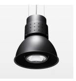
Suspended luminaire with LED, rated life of the LED L80/B10 > 50000 h, chromaticity tolerance 2 SDCM (initial), reflector with circular light distribution pattern, reflector pure aluminium 99,99% in MIRO-Silver®, luminaire shade die-cast aluminium, powder-coated, swivel angle +25°/-25°, luminaire housing sheet steel, powder-coated, stratoblack
