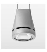
Suspended luminaire with LED, rated life of the LED L80/B10 > 50000 h, colour rendering index CRI > 80, chromaticity tolerance 2 SDCM (initial), reflector with circular light distribution pattern, reflector pure aluminium 99,99% in MIRO-Silver®, luminaire head die-cast aluminium, powder-coated, stratosilver
