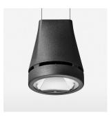
Suspended luminaire with LED, rated life of the LED L80/B10 > 50000 h, chromaticity tolerance 2 SDCM (initial), reflector with circular light distribution pattern, reflector pure aluminium 99,99% in MIRO-Silver®, luminaire head die-cast aluminium, powder-coated, stratoblack
