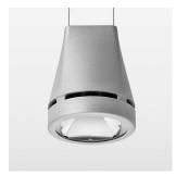
Suspended luminaire with LED, rated life of the LED L80/B10 > 50000 h, chromaticity tolerance 2 SDCM (initial), reflector with circular light distribution pattern, reflector pure aluminium 99,99% in MIRO-Silver®, luminaire head die-cast aluminium, powder-coated, stratosilver
