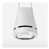
Suspended luminaire with LED, rated life of the LED L80/B10 > 50000 h, chromaticity tolerance 3 SDCM (initial), reflector with circular light distribution pattern, reflector pure aluminium 99,99% in MIRO-Silver®, luminaire head die-cast aluminium, powder-coated, stratowhite
