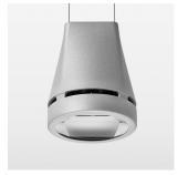
Suspended luminaire with LED, rated life of the LED L80/B10 > 50000 h, chromaticity tolerance 3 SDCM (initial), reflector with oval light distribution pattern, reflector pure aluminium 99,99% in MIRO-Silver®, luminaire head die-cast aluminium, powder-coated, stratosilver
