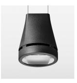
Suspended luminaire with LED, rated life of the LED L80/B10 > 50000 h, chromaticity tolerance 2 SDCM (initial), reflector with oval light distribution pattern, reflector pure aluminium 99,99% in MIRO-Silver®, luminaire head die-cast aluminium, powder-coated, stratoblack
