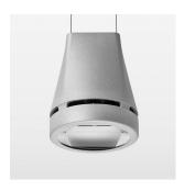
Suspended luminaire with LED, rated life of the LED L80/B10 > 50000 h, chromaticity tolerance 3 SDCM (initial), reflector with oval light distribution pattern, reflector pure aluminium 99,99% in MIRO-Silver®, luminaire head die-cast aluminium, powder-coated, stratosilver
