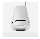
Suspended luminaire with LED, rated life of the LED L80/B10 > 50000 h, colour rendering index CRI > 80, chromaticity tolerance 2 SDCM (initial), reflector with oval light distribution pattern, reflector pure aluminium 99,99% in MIRO-Silver®, luminaire head die-cast aluminium, powder-coated, stratowhite
