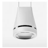
Suspended luminaire with LED, rated life of the LED L80/B10 > 50000 h, chromaticity tolerance 2 SDCM (initial), reflector with oval light distribution pattern, reflector pure aluminium 99,99% in MIRO-Silver®, luminaire head die-cast aluminium, powder-coated, stratowhite
