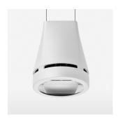
Suspended luminaire with LED, rated life of the LED L80/B10 > 50000 h, chromaticity tolerance 3 SDCM (initial), reflector with oval light distribution pattern, reflector pure aluminium 99,99% in MIRO-Silver®, luminaire head die-cast aluminium, powder-coated, stratowhite
