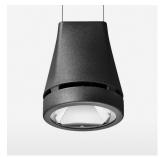
Suspended luminaire with LED, rated life of the LED L80/B10 > 50000 h, colour rendering index CRI > 80, chromaticity tolerance 2 SDCM (initial), reflector with circular light distribution pattern, reflector pure aluminium 99,99% in MIRO-Silver®, luminaire head die-cast aluminium, powder-coated, stratoblack
