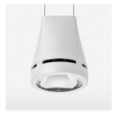
Suspended luminaire with LED, rated life of the LED L80/B10 > 50000 h, colour rendering index CRI > 80, chromaticity tolerance 2 SDCM (initial), reflector with circular light distribution pattern, reflector pure aluminium 99,99% in MIRO-Silver®, luminaire head die-cast aluminium, powder-coated, stratowhite
