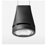
Suspended luminaire with LED, rated life of the LED L80/B10 > 50000 h, chromaticity tolerance 2 SDCM (initial), reflector with circular light distribution pattern, reflector pure aluminium 99,99% in MIRO-Silver®, luminaire head die-cast aluminium, powder-coated, stratoblack
