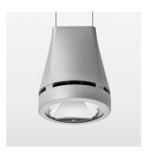
Suspended luminaire with LED, rated life of the LED L80/B10 > 50000 h, chromaticity tolerance 2 SDCM (initial), reflector with circular light distribution pattern, reflector pure aluminium 99,99% in MIRO-Silver®, luminaire head die-cast aluminium, powder-coated, stratosilver
