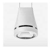
Suspended luminaire with LED, rated life of the LED L80/B10 > 50000 h, chromaticity tolerance 3 SDCM (initial), reflector with circular light distribution pattern, reflector pure aluminium 99,99% in MIRO-Silver®, luminaire head die-cast aluminium, powder-coated, stratowhite
