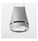
Suspended luminaire with LED, rated life of the LED L80/B10 > 50000 h, colour rendering index CRI > 90, chromaticity tolerance 2 SDCM (initial), reflector with circular light distribution pattern, reflector pure aluminium 99,99% in MIRO-Silver®, luminaire head die-cast aluminium, powder-coated, stratosilver
