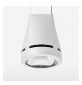
Suspended luminaire with LED, rated life of the LED L80/B10 > 50000 h, colour rendering index CRI > 80, chromaticity tolerance 2 SDCM (initial), reflector with circular light distribution pattern, reflector pure aluminium 99,99% in MIRO-Silver®, canopy sheet steel, powder-coated, luminaire head die-cast aluminium, powder-coated, stratowhite
