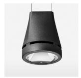
Suspended luminaire with LED, rated life of the LED L80/B10 > 50000 h, colour rendering index CRI > 80, chromaticity tolerance 2 SDCM (initial), reflector with circular light distribution pattern, reflector pure aluminium 99,99% in MIRO-Silver®, canopy sheet steel, powder-coated, luminaire head die-cast aluminium, powder-coated, stratoblack
