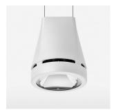
Suspended luminaire with LED, rated life of the LED L80/B10 > 50000 h, colour rendering index CRI > 80, chromaticity tolerance 2 SDCM (initial), reflector with circular light distribution pattern, reflector pure aluminium 99,99% in MIRO-Silver®, canopy sheet steel, powder-coated, luminaire head die-cast aluminium, powder-coated, stratowhite
