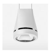
Suspended luminaire with LED, rated life of the LED L80/B10 > 50000 h, chromaticity tolerance 3 SDCM (initial), reflector with circular light distribution pattern, reflector pure aluminium 99,99% in MIRO-Silver®, canopy sheet steel, powder-coated, luminaire head die-cast aluminium, powder-coated, stratowhite
