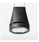
Suspended luminaire with LED, rated life of the LED L80/B10 > 50000 h, colour rendering index CRI > 90, chromaticity tolerance 2 SDCM (initial), reflector with circular light distribution pattern, reflector pure aluminium 99,99% in MIRO-Silver®, canopy sheet steel, powder-coated, luminaire head die-cast aluminium, powder-coated, stratoblack
