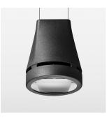
Suspended luminaire with LED, rated life of the LED L80/B10 > 50000 h, colour rendering index CRI > 80, chromaticity tolerance 2 SDCM (initial), reflector with oval light distribution pattern, reflector pure aluminium 99,99% in MIRO-Silver®, canopy sheet steel, powder-coated, luminaire head die-cast aluminium, powder-coated, stratoblack
